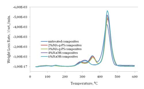
Fig.4: The DTG curve of the untreated and treated SPF-HIPS composites
